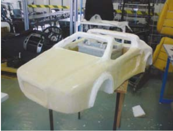
7. Mockup fabrication (scale 1:4)
