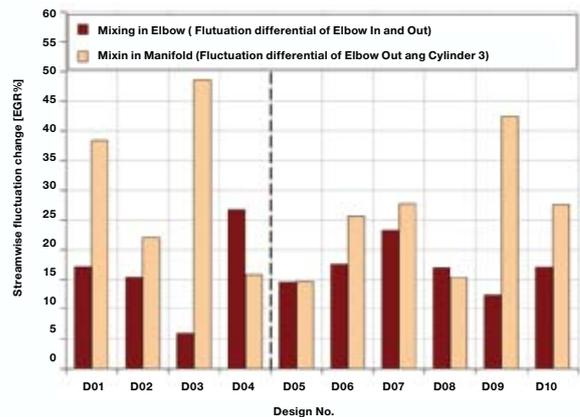
Figure 17. Contribution to EGR rate fluctuation (B vehicle)
