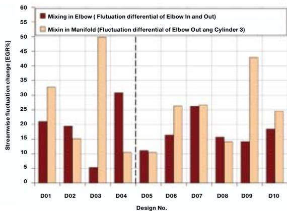
Figure 16. Contribution to EGR rate fluctuation (A vehicle)
